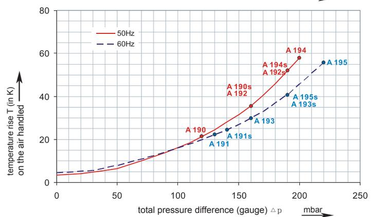
The performance curves are based on air at a temperature of 15 °C and an atmospheric pressure of 1013 mbar with a tolerance of +/- 10 %.
