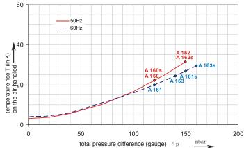
The performance curves are based on air at a temperature of 15 °C and an atmospheric pressure of 1013 mbar with a tolerance of +/- 10 %. The total pressure differences are valid for suction and ambient temperatures up to 25 °C.
