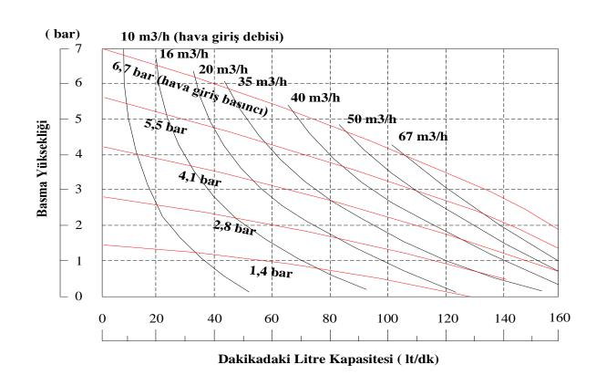
Suction / Discharge 1" Max. Capacity 160 lpm Max. Solid particle (4 mm) Max. Operation pressure 8,4 bar Weight 9 kg (AL)
