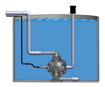
Diaphragm pumps can also be used as submerged pump. It is necessary to maintain the exhaust port of the pump above the liquid surface with pipe or hose.
